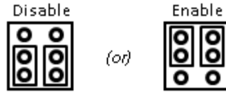
Figure 3 – J1939 TERM Jumper Setting
