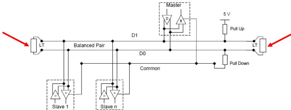
LT = Line Termination 120-ohm resistor
