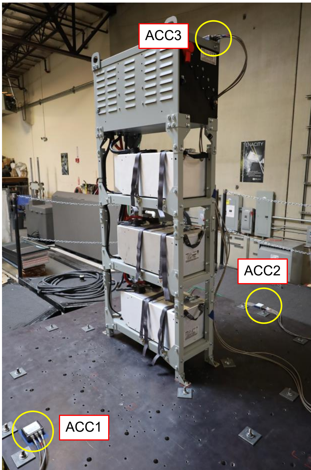
Figure C.7. UUT-01 accelerometer ACC1, ACC2 and ACC3 locations.
