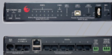
Front and review view of LED's and available ports.
