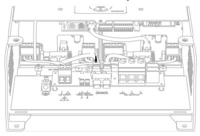
**S4 Ground Fault Jumper**
