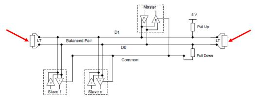
LT = Line Termination 120-ohm resistor
