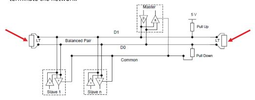
LT = Line Termination 120-ohm resistor
