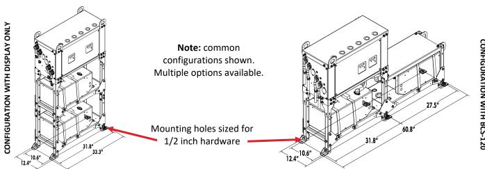
5.1.6. Allow sufficient room for routing the fixed wiring to the system. Alarm and communications field connections may enter the optional termination panel using conduit knockouts.
