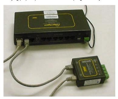
in this illustration the ROM is connected to the SC4 Site Controller.
