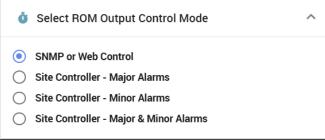
Selecting any of the three options above will allow you to control the output state by whether an alarm is present or not for that specific option. After selecting one of these three options you'll notice a box will appear below (shown below) that will allow you to select individual string or jar level alarm(s) that will change the output.
