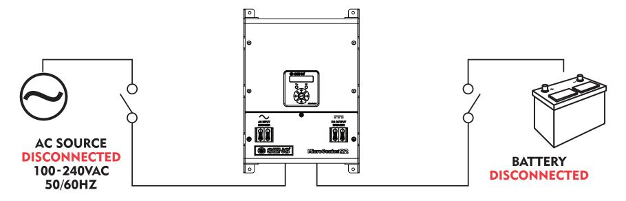
Note - Chargers configured to boost may be in boost for up to 24 hours at start-up if battery voltage is low
