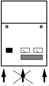
WHEN INSTALLING DO NOT LIFT UNIT FROM MIDDLE OF LOWER COVER - THE COVER WILL BEND.
