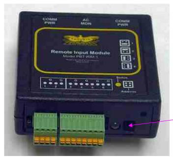
Remove the jumper by pulling it straight out. Replace the jumper in one of the 4 positions shown on the RIM label to set the address. The jumper should always connect 2 pins on the address header. The RIM will not operate properly if an address jumper is not installed.
