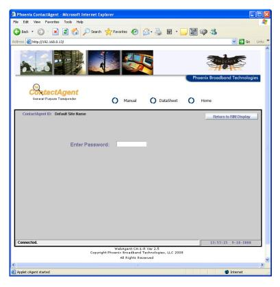
Type the password followed by enter. The password is case sensitive. There are two passwords, one for User access and one for Administrative access. The default passwords are "user" and "admin". The passwords can be changed from the telnet setup interface on the Host device ( $ContactAgent^{TM}$ ).
