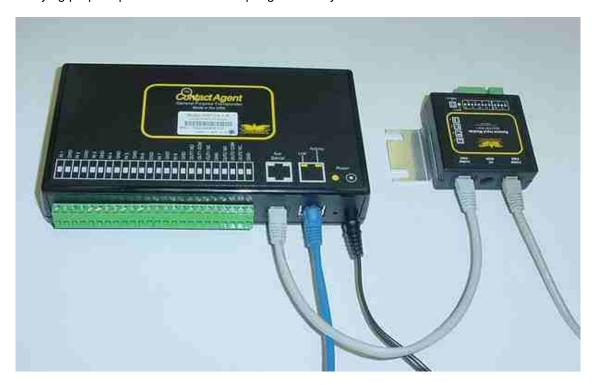
Connect the Aux Serial port on the *ContactAgent*™ to either "COMM/PWR" port on the RIM. Connect the other "COMM/PWR" port on the RIM to the next PBT Remote Module. Up to 4 RIMs with different address settings may be connected in a daisy chain with ROMs or other compatible PBT devices.
