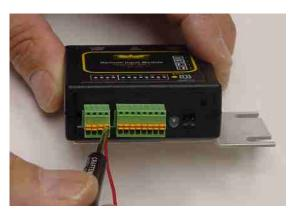
To remove a wire from the barrier block press the orange release button with a small screw driver and pull the wire free.
