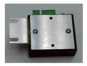
The hole spacing in the bracket is designed to fit a 1U space on an equipment rack rail. The bracket can be secured to a rack rail using customer provided hardware appropriate for
