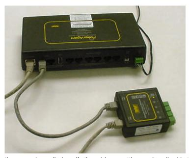
in this illustration the ROM is connected to the SC3 Site Controller.
