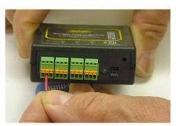
accommodate 20-26 AWG wire. Strip 0.25 inch of insulation from the wire. Solid wire works best, but if you use stranded wire be sure to twist the strands tightly together. Push the wire into the desired barrier block connection as shown. There is common, normally open and normally closed connection for each output.
