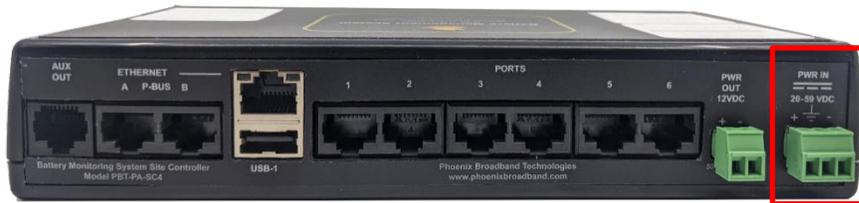
PWR IN Connector – Shown from Rear Panel of SC4
