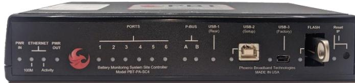
The Site Controller front panel has numerous indicators for quick assessment of power, connection status, and network connectivity.
