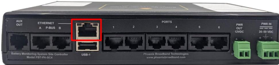
The Genset BMS ships with a 25-foot CAT5 cable (PBT-PAC-CAT5-25) connected to this port and spooled inside the cabinet.
