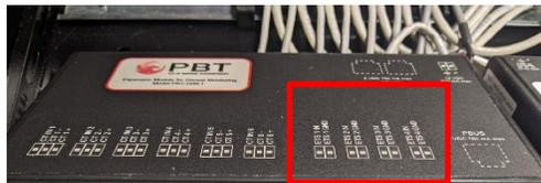
6. Lightly tug the leads to ensure that they are locked in and installed properly.
