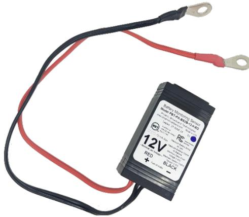
Each sensor continuously monitors the voltage and temperature of the connected jar. At user-defined intervals, the sensor measures the jar admittance by generating a digitally synthesized AC test signal of approximately 0.5 to 6.0 amps, which drives the jar's terminals for testing purposes. This test current causes a small AC voltage, proportional to jar impedance. This voltage is sampled by the sensor to determine the jar's internal AC impedance, which is the basis for admittance measurements.
