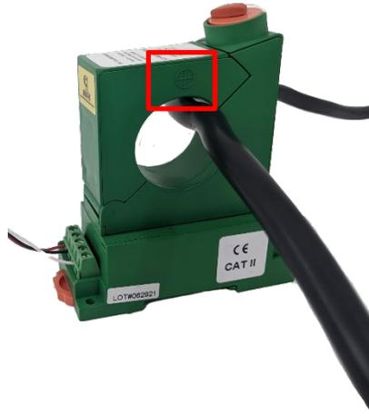
3. Unspool one of the current sensor cables from the PBT-GIM-1 and fish the cable from the cabinet.
